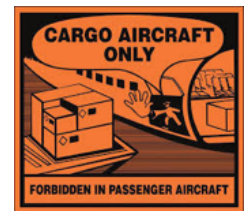
Figure 3. Label indicating a shipment can only be carried on a cargo aircraft (CAO) following UN3480-PI965 Section II.
