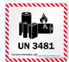
Figure 4. Li-ion battery label for shipping either batteries packed with or in equipment under UN3481-PI966 or PI967.
