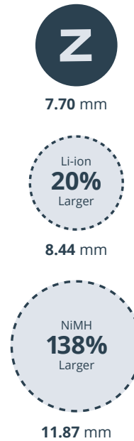
Figure 2. Battery diameters and relative sizes required to deliver 58 mWh of energy given a cell height of 3.35mm (size XR41) in 2019.
